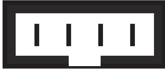
Figure 4-3: J4 - RS-232 Jack Pinout
